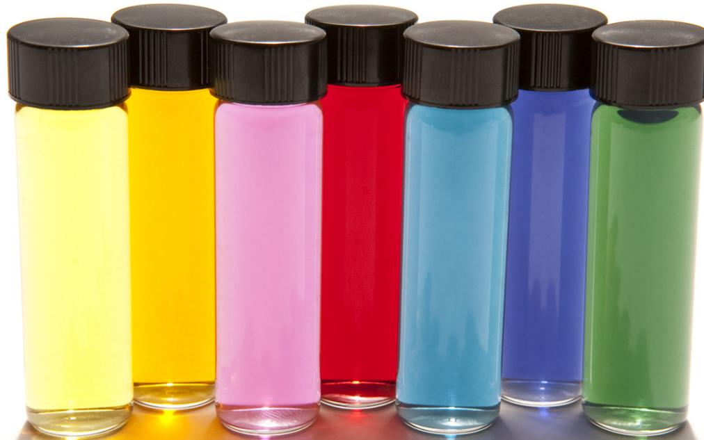
Optical response of metal nanoparticles is a function of the material, size, shape and local environment
